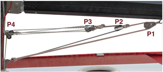
The vang fitting is installed as standard on the boom 7 60 cm from the gooseneck bolt on the mast. The fitting should have one side bolted into a hole drilled into the underside of the boom - if just friction is used then the fitting tends to creep towards the mast under tension
