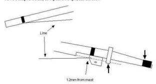
Measure the distance between line and the markers on the mast. Make sure you measure at a right angle to the line. Measure also the difference in vertical
