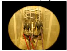
3 - Fix 4 double pulley-bulkhead, two each side of the centercase.
