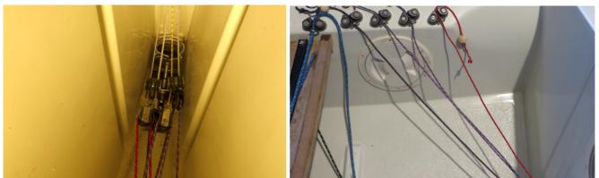
• On the left of the diagram (in red) the control line passes from the side deck, through a pulley in the forward bulkhead, through the pulley of the line passing around the mast foot, back through the pulley on the bulkhead and to the other side in a symmetric fashion.
