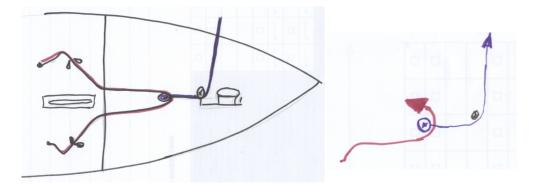
Each control line has two parts. In blue (on the right of the diagram) an end passes through one of the pulleys fixed to the base of the mast and passes backwards to a small pulley, generally Ø16 - 22 mm.
